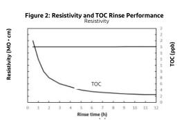
$<sup>^{\</sup>ddagger}$  Based on 18.2-M $\Omega$ - cm feedwater. AmberTec<sup>TM</sup> UP6040 H/OH will deliver 18.2 M $\Omega$ - cm quality water with total organic carbon levels well below 1 ppb, in well-designed UPW systems.
