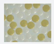
The ratio of anion to cation in AmberTec™ MR-300 UPW H/OH is volumetrically optimized to achieve maximum removal of boron and silica.
