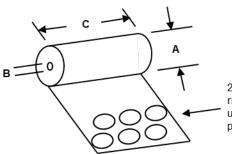
2 x 8.0"-diameter left, center, right Plate & Frame samples used to determine nominal performance of the roll.
